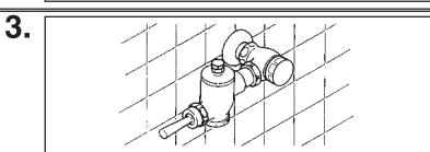
Insert the flushometer valve tailpiece ® into the stop valve A and hand tighten the lock nut D to the stop valve. Plumb the entire unit.
